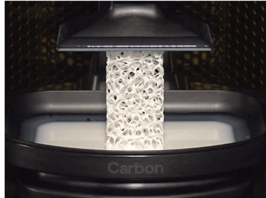
*Using Carbon Digital Light Synthesis technology, small and complex parts “grow” out of a reservoir of UV-curable liquid resin.*
